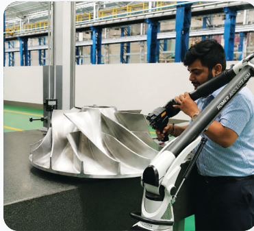
Final Inspection of New Impeller
