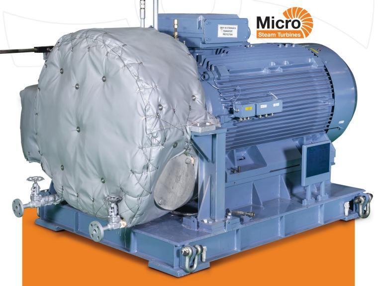
Triveni Turbines offers SMART (Sustainable Modularly Arranged Pressure Reducing Turbine) units, which are essentially backpressure steam turbines. These units perform the same function as **pressure-reducing** stations while simultaneously generating **additional electricity** by converting steam energy into electrical energy.
