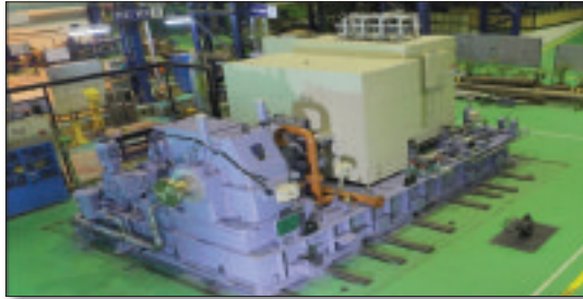
Fig 1 30MW Extraction condensing steam turbine
