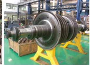
TRIVENI ROTOR WITH 9 STAGES (BACK PRESSURE DESIGN)
