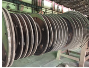
OEM ROTOR WITH 17 STAGES (CONDENSING DESIGN)
