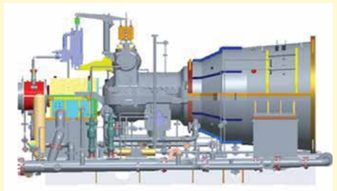
Figure 1: Axial exhaust turbine with controlled extraction for sugar factory cogeneration
