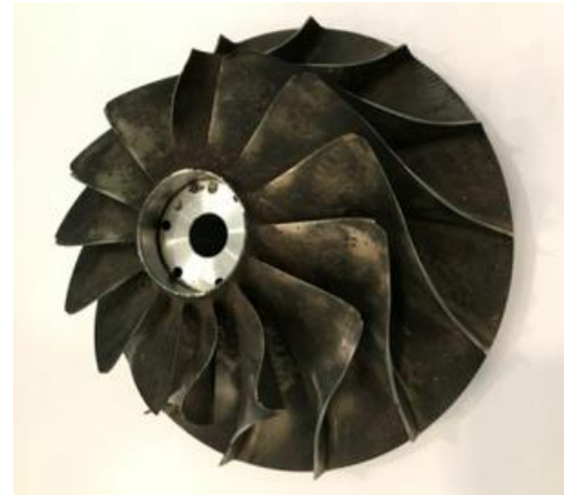
Old damaged Impeller
