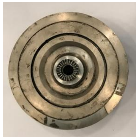
Old damaged Impeller – Hirth teeth side
