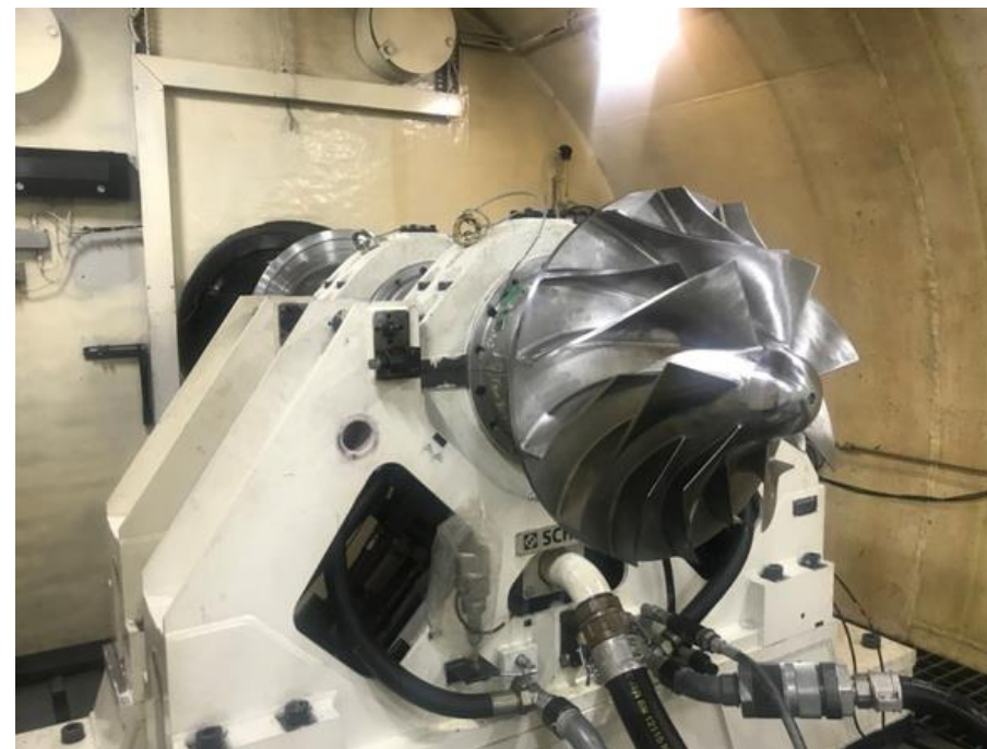
Final Assembly of the Impeller with new pinion shaft and Balancing setup
