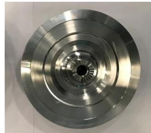
New Impeller - Hirth teeth side
