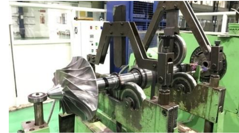
Final Assembly of the Impeller with new pinion shaft and Balancing setup
