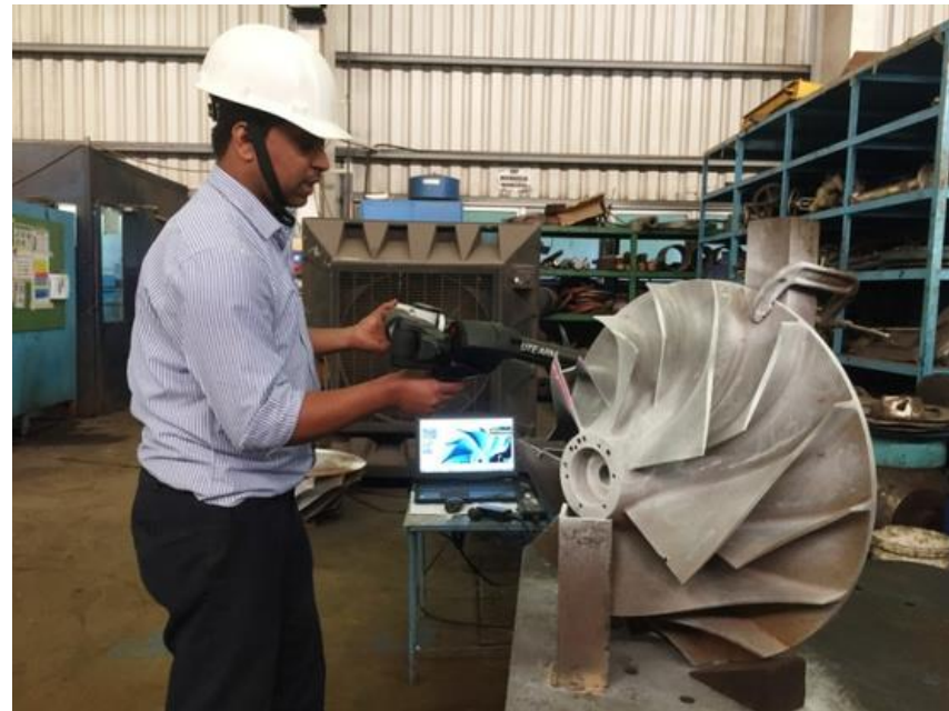
Reverse engineering of damaged Impeller at site
