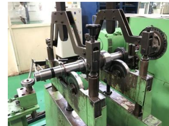
Manufactured new pinion shaft and individual Balancing setup
