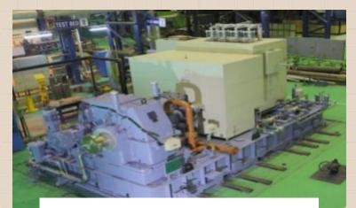
The project is driven by 30 MWe extraction condensing steam turbine with an inlet steam pressure of 65 Bar and inlet temperature of 490 Deg C
