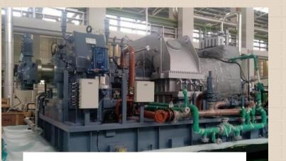
The project is driven by 1\*30 MWe Bleed condensing steam turbines with an inlet steam pressure of 65 Bar and 505 Deg C with 0.1 Bar Exhaust pressure
