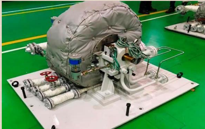
The project is driven by 12 No's of steam turbines for various pump units as per API 611 for an Oil Refinery in North America
