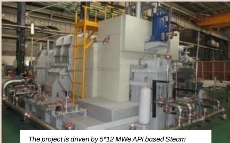
The project is driven by 5*12 MWe API based Steam Turbine for an Oil Refinery in India
