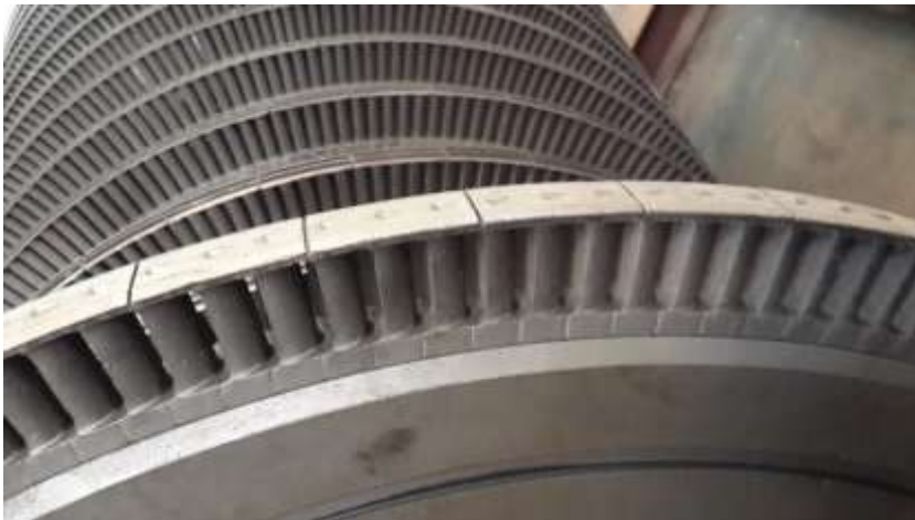
Damages to the rotor blades due to corrosion and age
