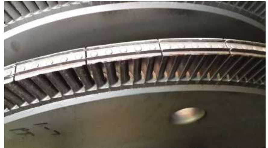
Damages to the rotor blades due to corrosion and age
