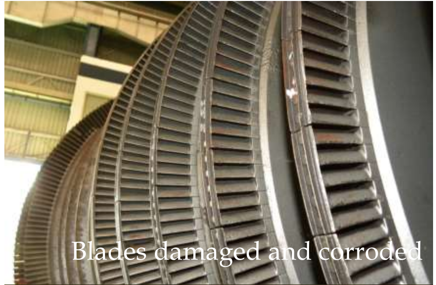
Fins badly damaged
